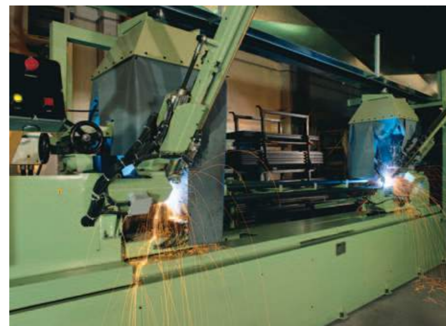
Automatic machine for welding Multiceta cross braces.
