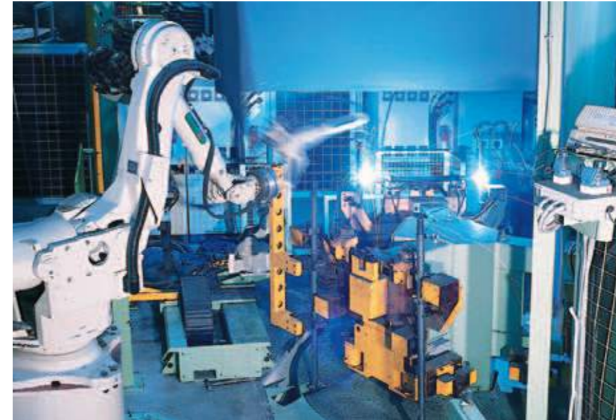
Automated island for welding frames.
